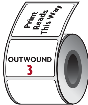
3. Copy is printed Around the roll. Right Side of the label comes off first.
