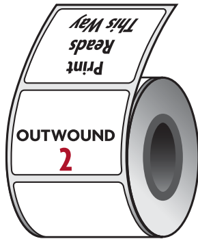
2. Copy is printed Across the roll. Bottom of the label comes off first.
