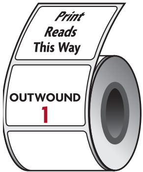
1. Copy is printed Across the roll. Top of the label comes off first.
