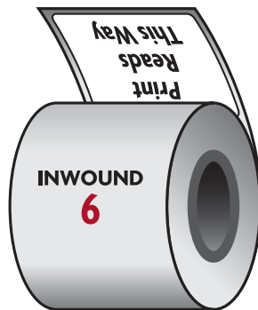
6. Copy is printed Across the roll. Bottom of the label comes off first.
