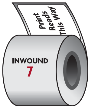
7. Copy is printed Around the roll. Right Side of the label comes off first.
