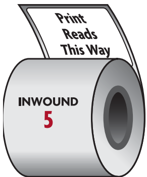
5. Copy is printed Across the roll. Top of the label comes off first.
